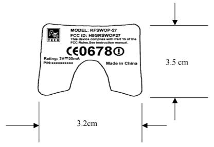
The remained portion of label statement required by FCC is attached in the user's manual.
