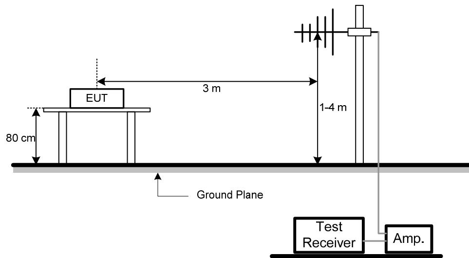
Radiated Emission Test Set-Up Frequency Above 1 GHz
