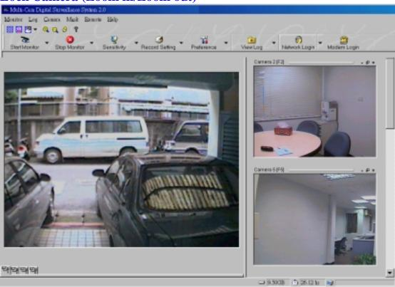
You can select any one of the camera to Zoom in or Zoom out, just press the icon between "-" and "x" or press the function key F1 to F6, F1 represent to camera 1. You can press the tool bar icon to zoom in or zoom out, or use the numeric keypad "-", "+". You can press the ESC key to back to the default display status.
