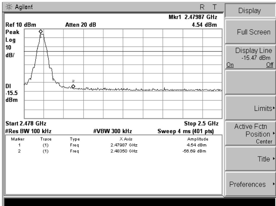
**Hopping On - ( $\pi/4$ DQPSK)**
