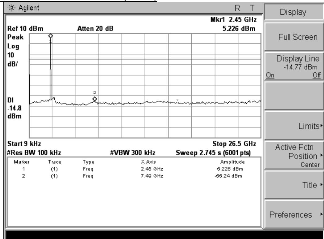
**9KHz-25GHz High Channel(GFSK)**
