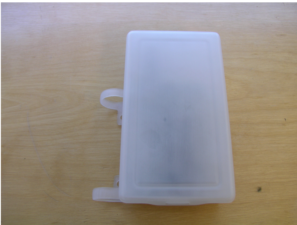
Test setup photos show the device in the old enclosure(case). The case has been changed in order to fully contain the antenna in the enclosure.
