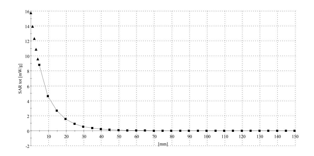
900 MHz System Performance Check / Dipole Sn# 96
