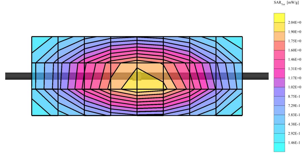
900 MHz System Performance Check / Dipole Sn# 96
