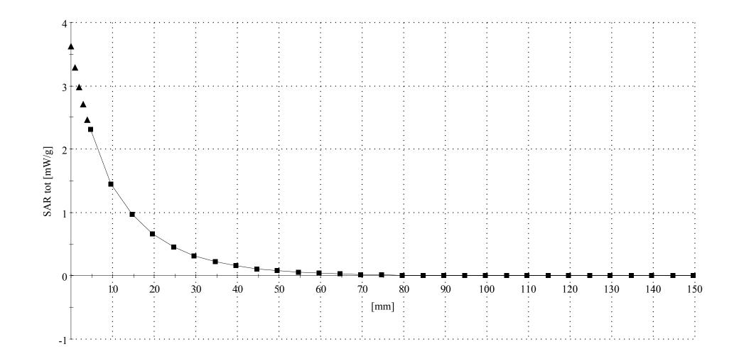
1800MHz System Performance Check / Dipole Sn# 272tr
