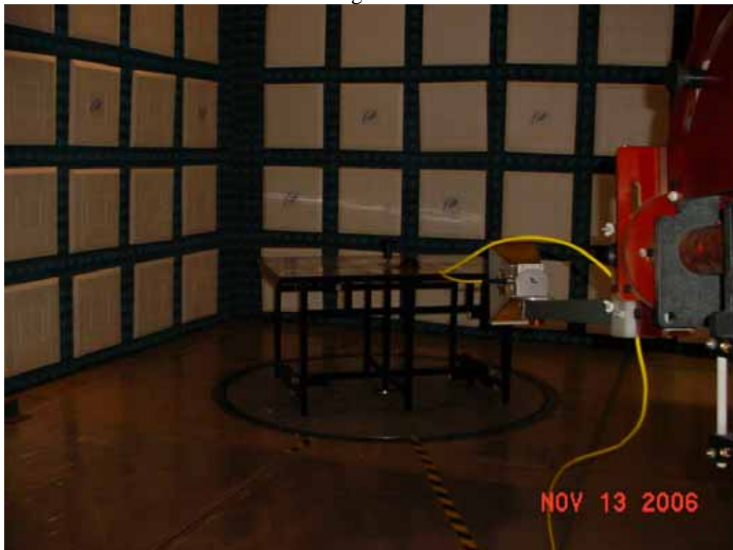
Test Setup for Radiated Emissions, 1GHz to 10GHz, with no metal enclosure – Horizontal Polarization
