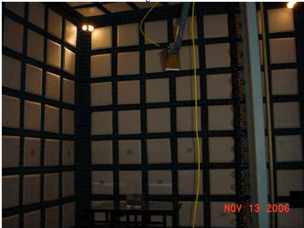
Test Setup for Radiated Emissions, 1GHz to 10GHz, with metal enclosure – Horizontal Polarization
