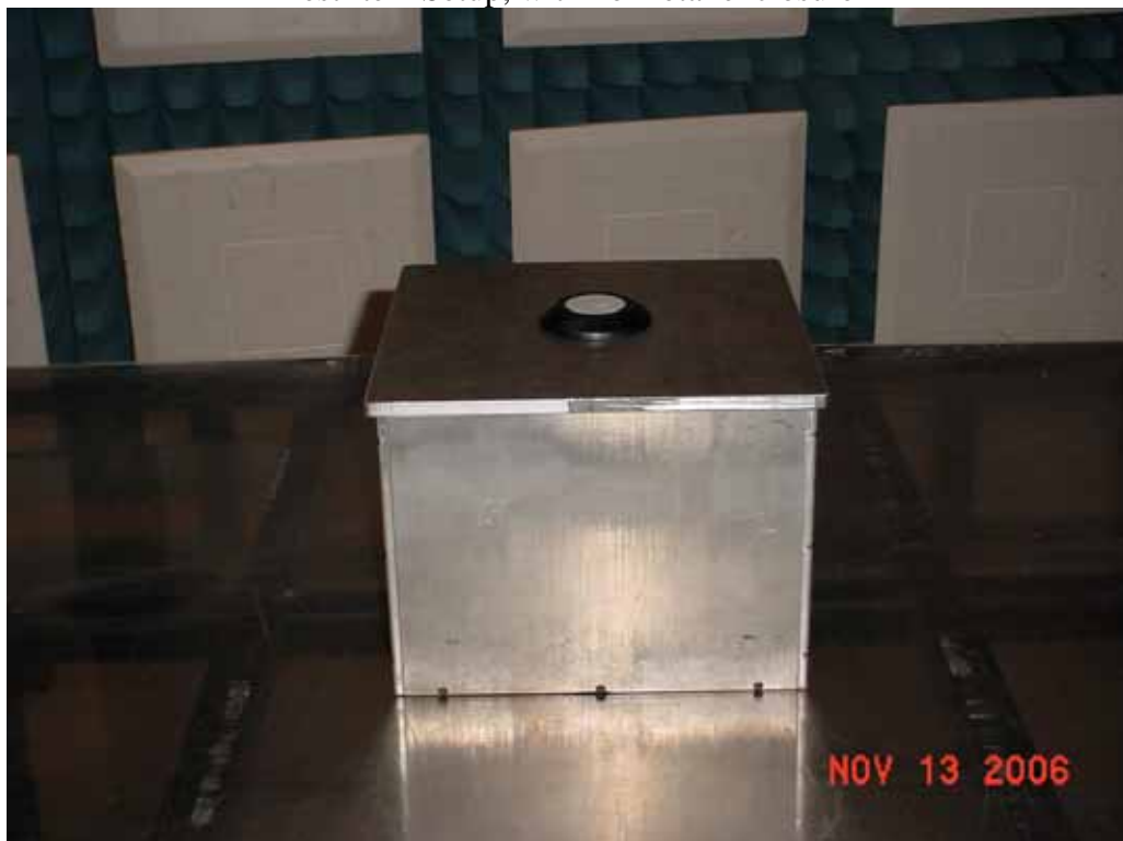
Test Item Setup, with metal enclosure
