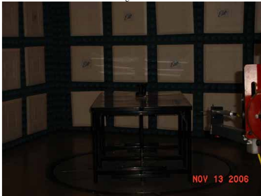
Test Setup for Radiated Emissions, 916.45MHz, with no metal enclosure – Horizontal Polarization
