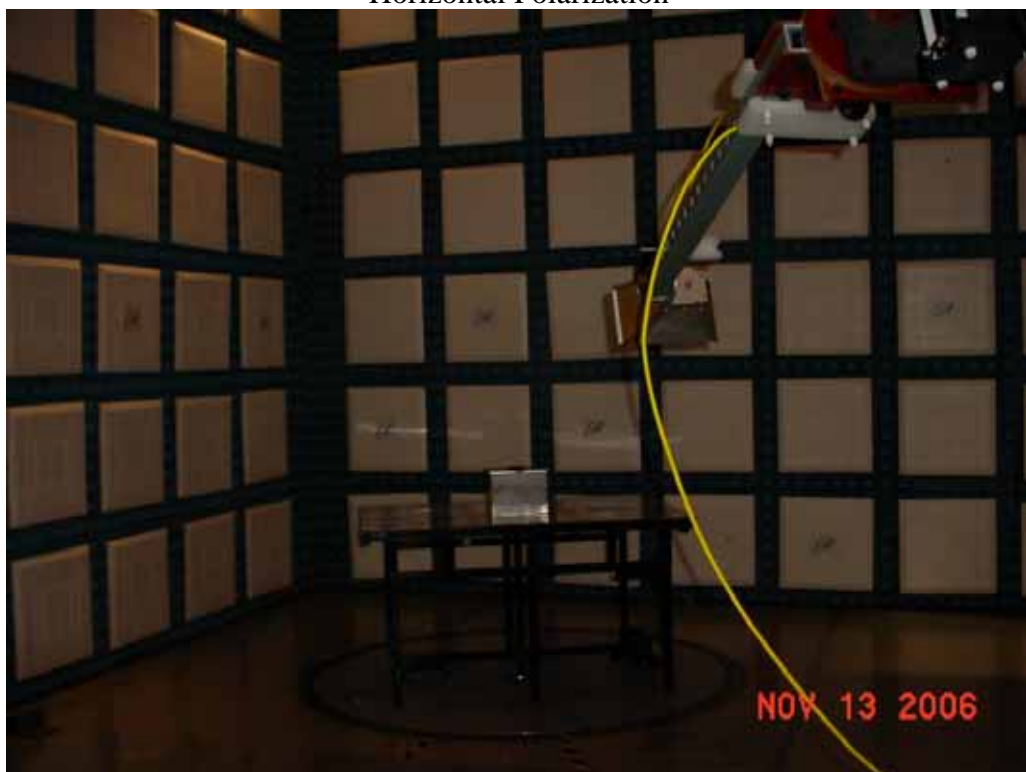
Test Setup for Radiated Emissions, 1GHz to 10GHz, with metal enclosure – Vertical Polarization
