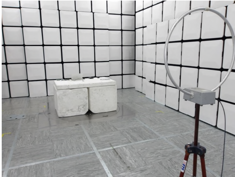
Photo 1.5-1 – Front View of the Test Setup, 3m - Out of band emissions below 30MHz
