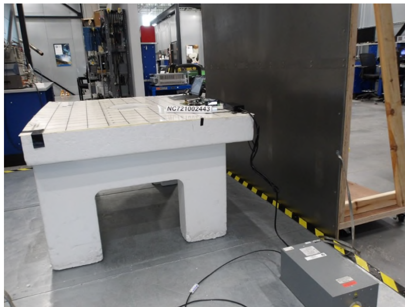
Photo 1.2-2 – Conducted Emission Test Setup [Front View]
