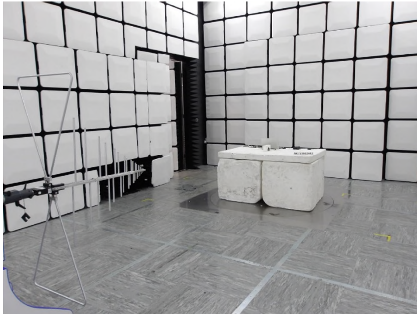
Photo 1.5-3 – Front View of the Test Setup, 3m - Out of band emissions 30 - 1000MHz
