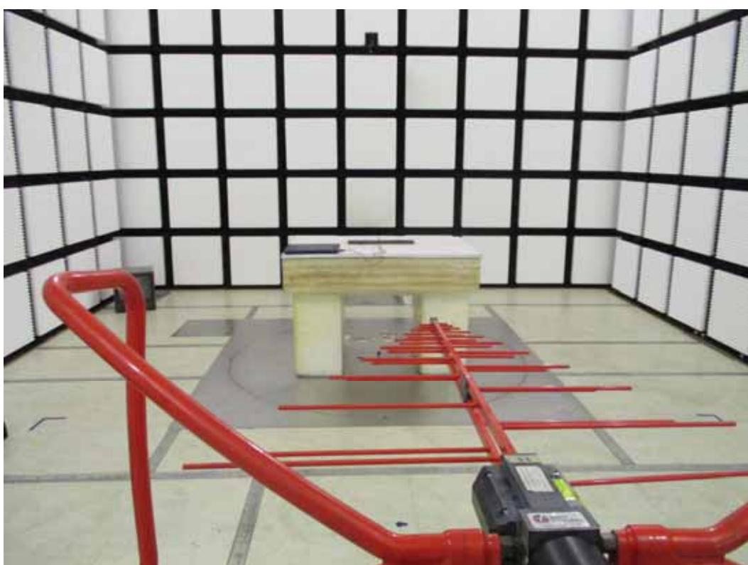
**RADIATED RF MEASUREMENT SETUP**
