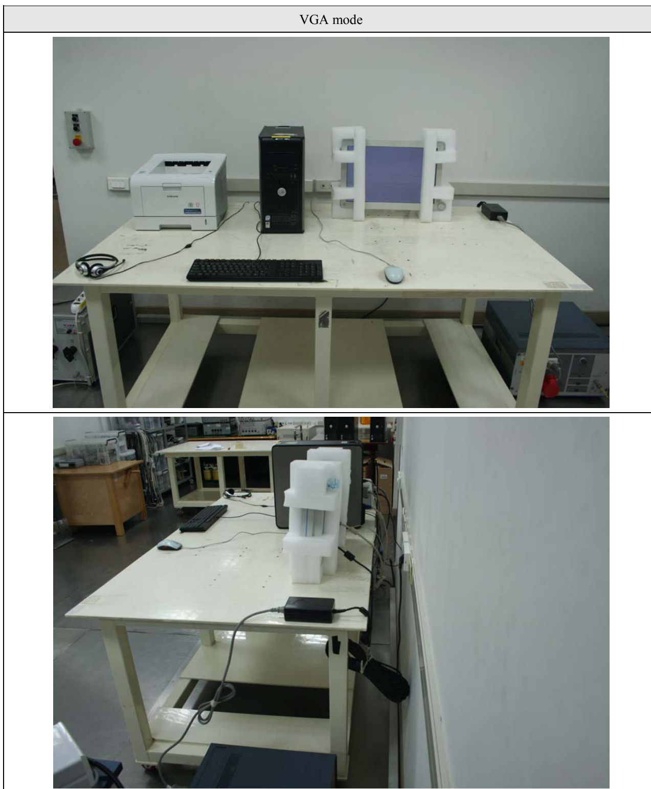
Figure 1. Conducted Emission Test Setup
