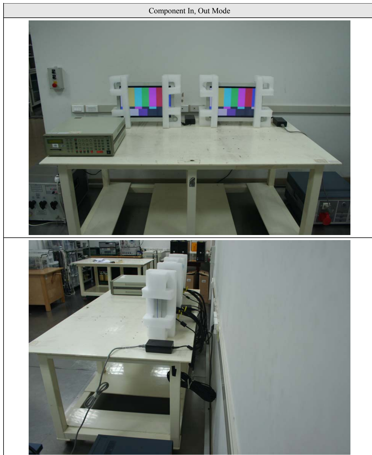
Figure 2. Conducted Emission Test Setup
