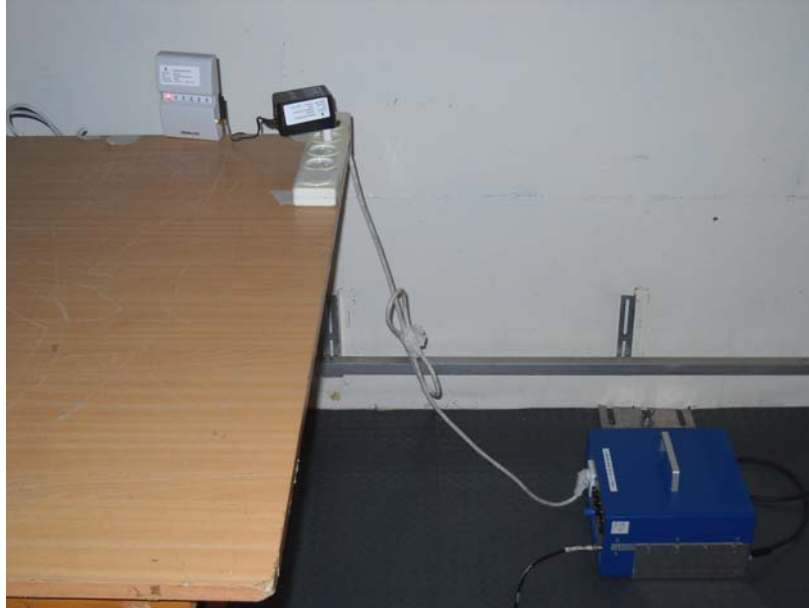
Photograph No.7 Setup for conducted emission measurements on AC power lines
