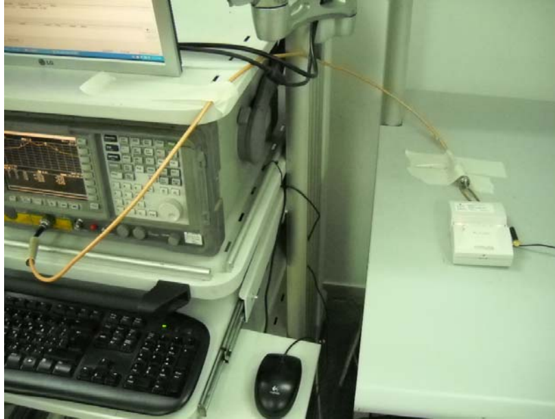
Photograph No.6 Setup for occupied bandwidth measurements
