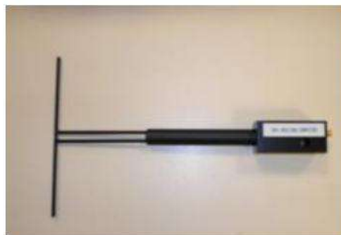
Figure 1 – Satimo COMOSAR Validation Dipole
