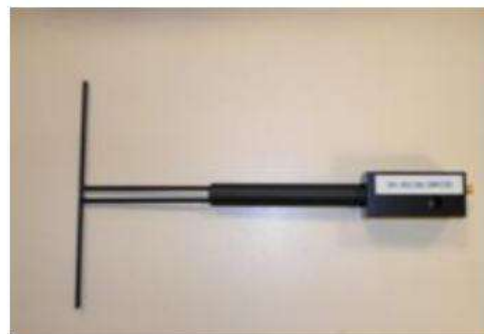
Figure 1 – Satimo COMOSAR Validation Dipole
