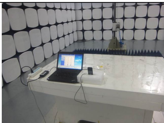
Radiated Spurious Emissions Test Setup Above 1GHz
