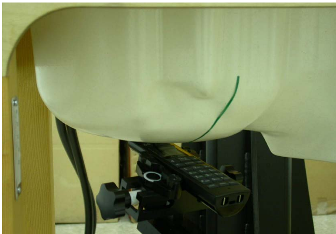
Measurement Position of Right-Tilt (RT) with Handset
