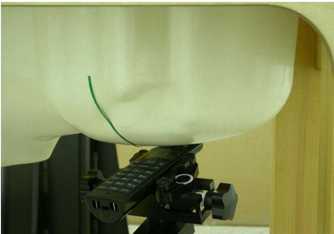
Measurement Position of Left-Tilt (LT) with Handset
