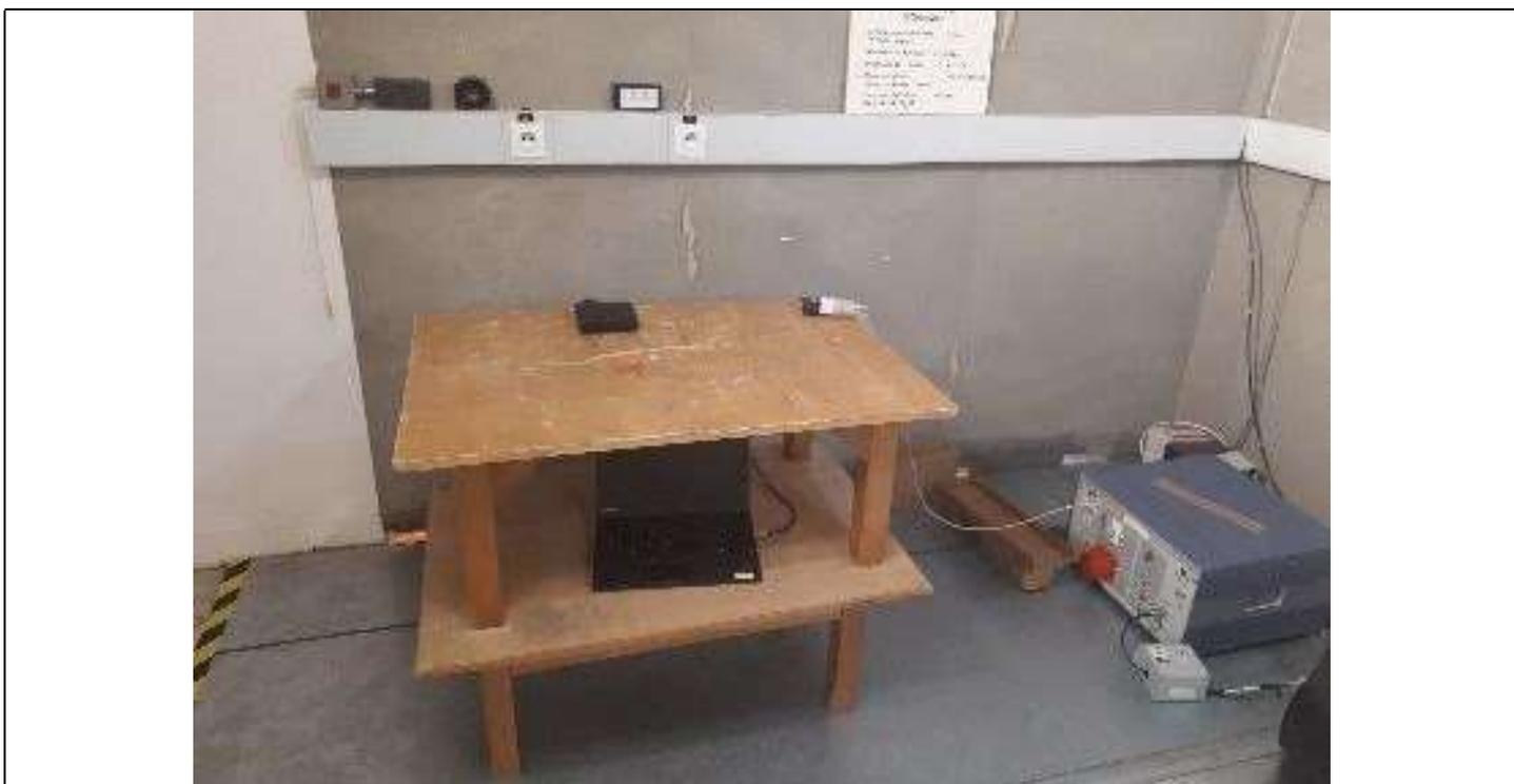
Photograph for AC Power Line Conducted Emission (Front view)
