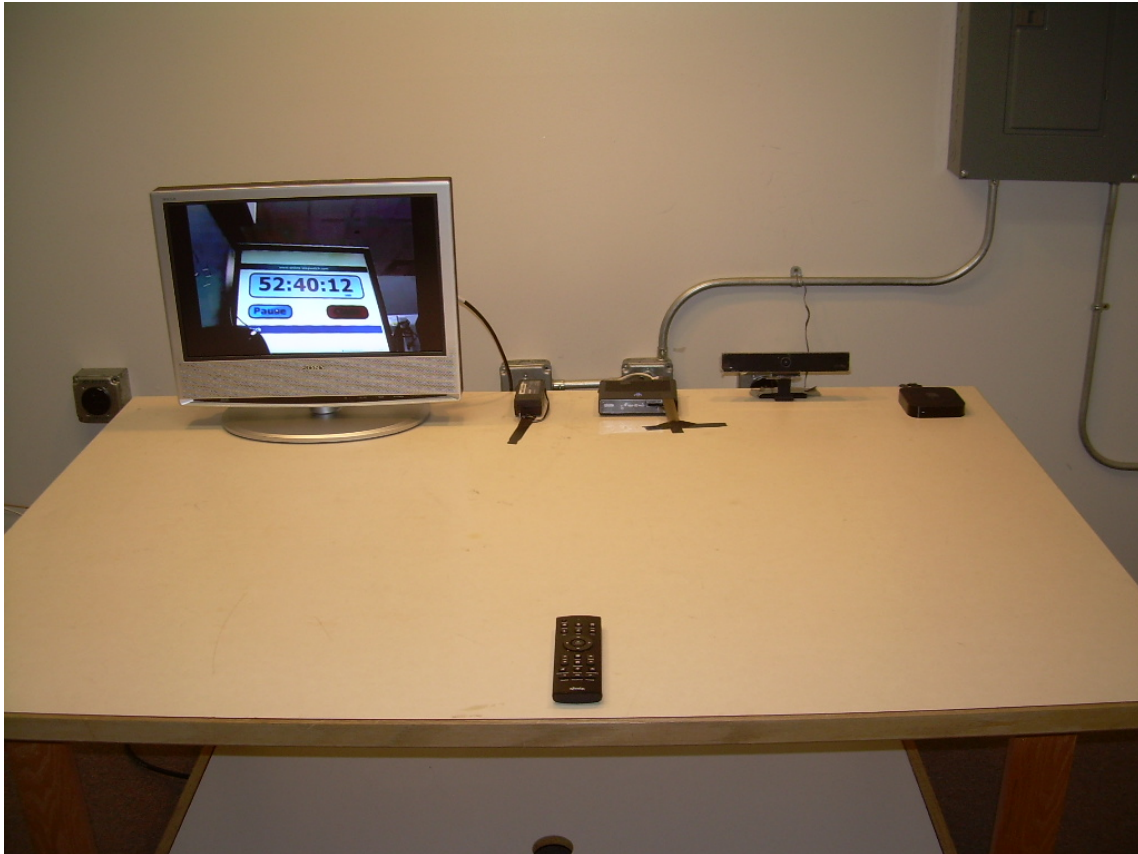
Photograph 3 – Front View Conducted Disturbance Test Configuration
