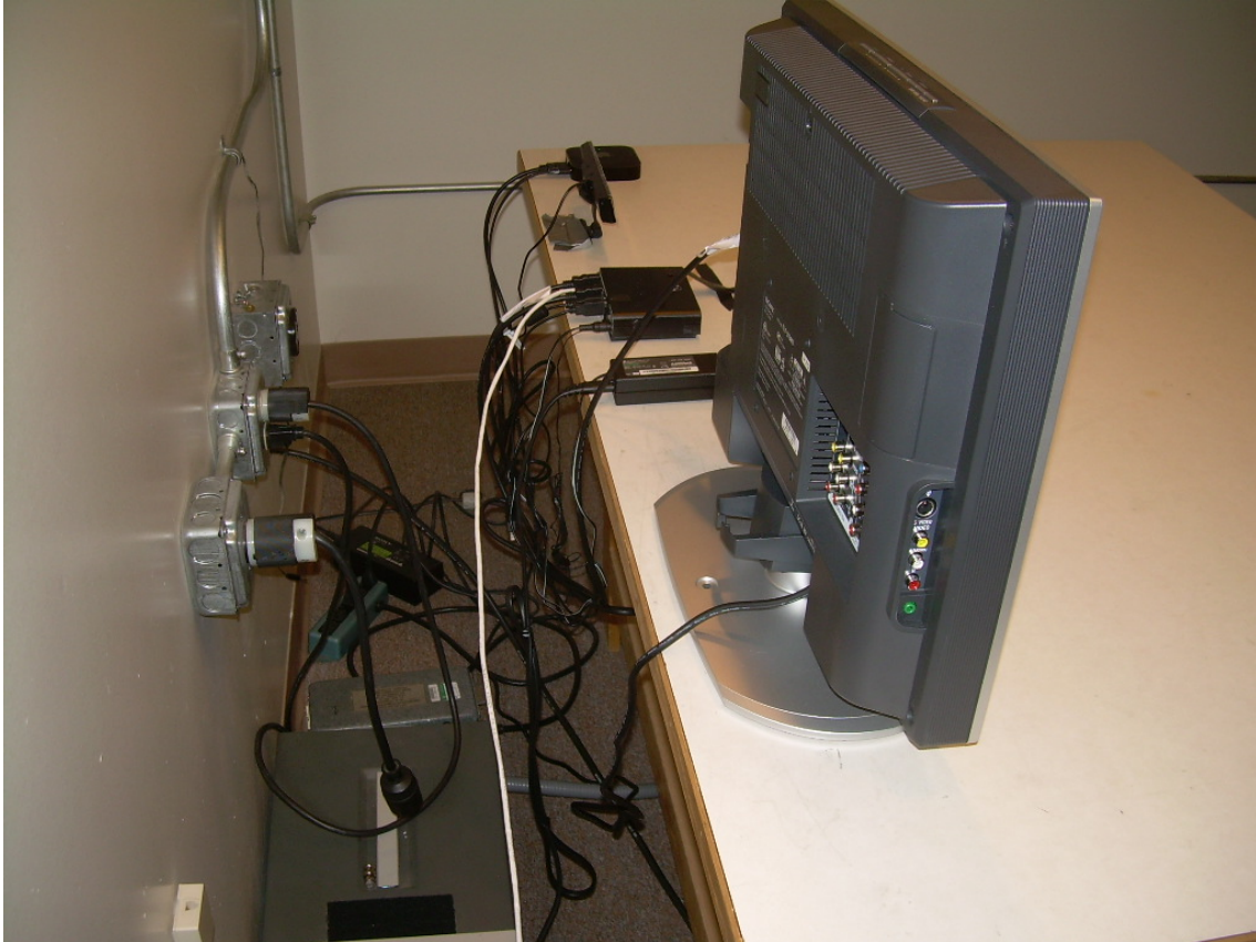
Photograph 4 – Back View Conducted Disturbance Test Configuration
