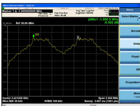
(1Mbps) Channel Separation plot on channel 39-40
