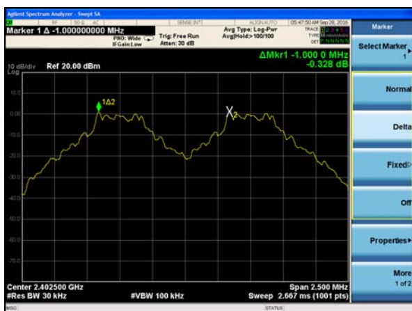
(1Mbps) Channel Separation plot on channel 39-40
