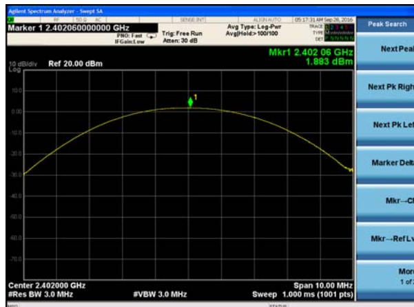
Peak output Power plot on channel 39 (2Mbps)
