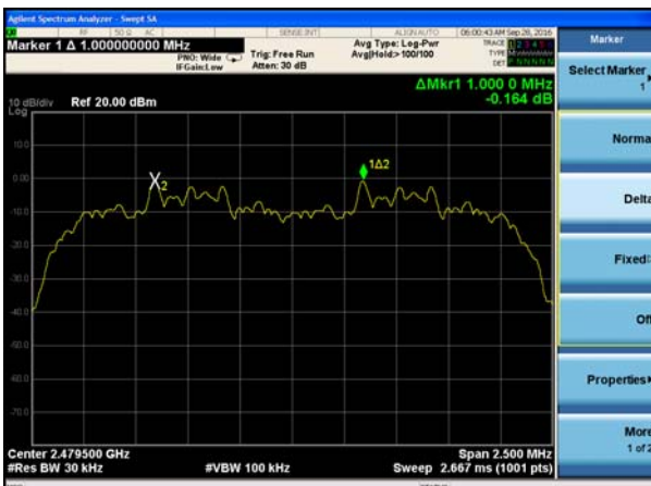
(2Mbps) Channel Separation plot on channel 77-78
