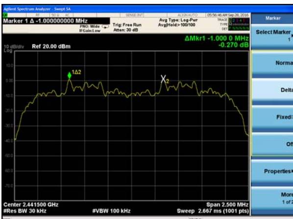
(2Mbps) Channel Separation plot on channel 39-40
