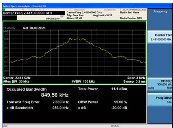
20dB Bandwidth plot on channel 78 (1Mbps)
