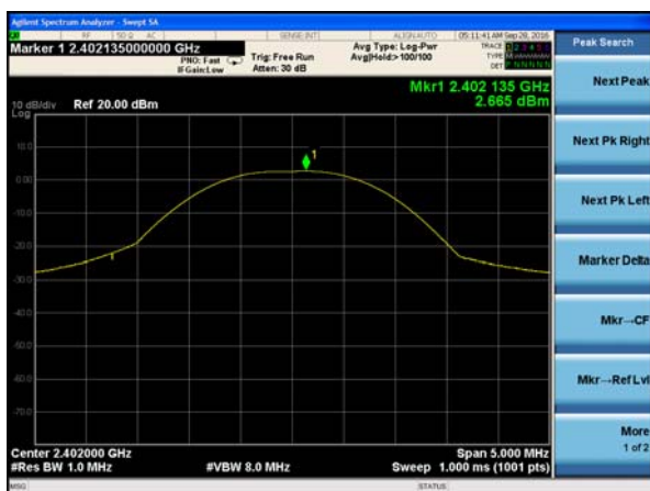
Peak output Power plot on channel 39 (1Mbps)
