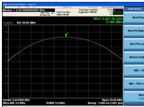
Peak output Power plot on channel 39 (2Mbps)
