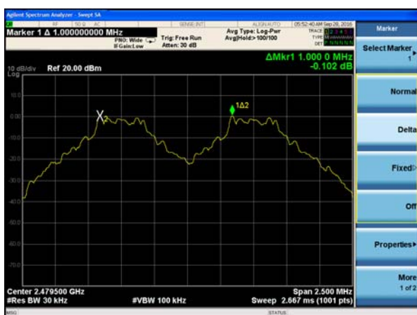
(1Mbps) Channel Separation plot on channel 77-78
