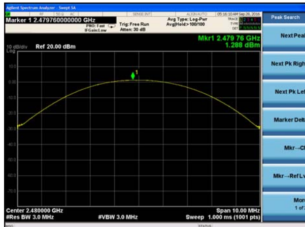
Peak output Power plot on channel 78 (2Mbps)
