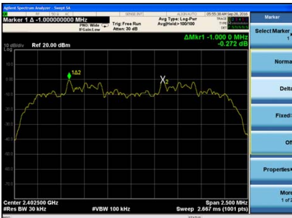
(2Mbps) Channel Separation plot on channel 39-40
