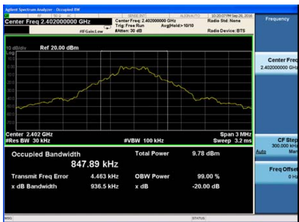
20dB Bandwidth plot on channel 39 (1Mbps)
