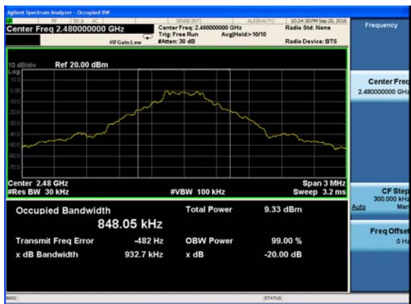
20dB Bandwidth plot on channel 78 (1Mbps)
