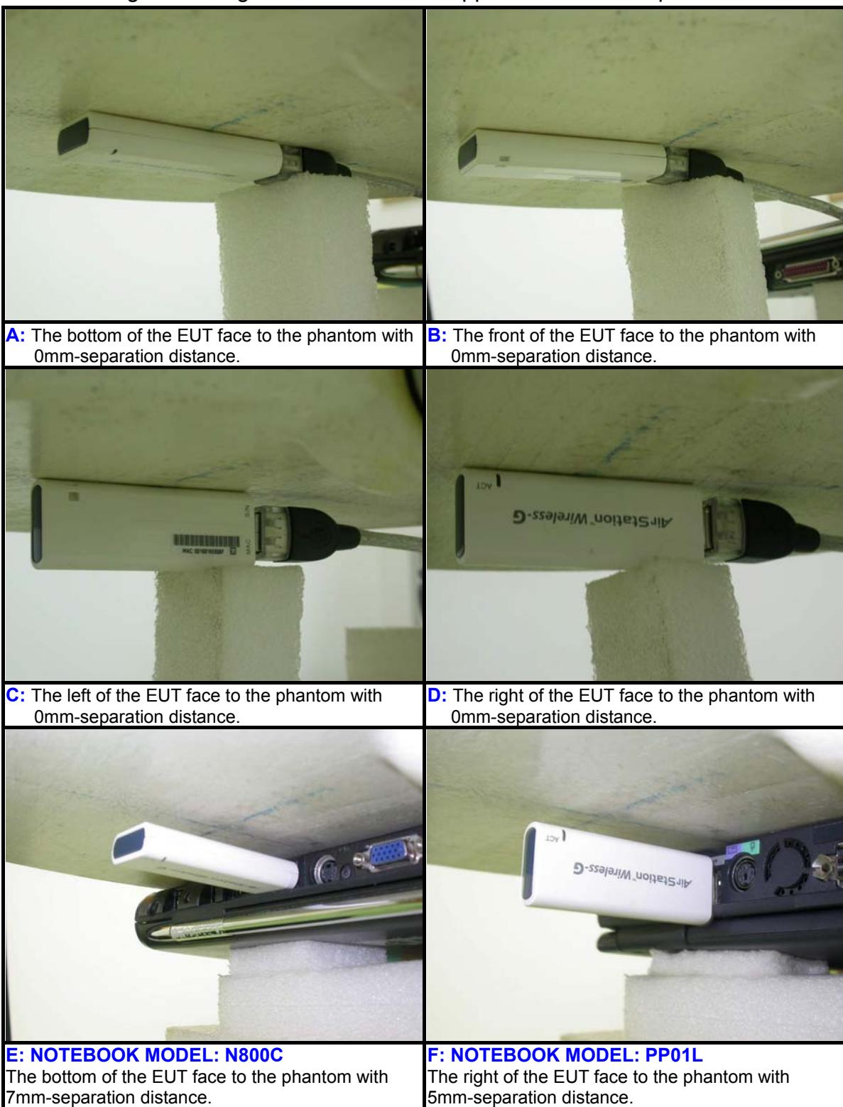
**NOTE:** The bottom of the notebook contacts the bottom of the flat phantom with 0mm-separation distance.
