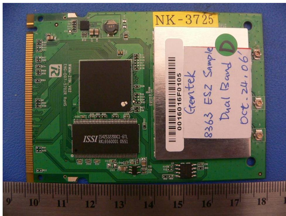
**EUT – RF Board Dual Band without RF Shielding (Component Side View)**
