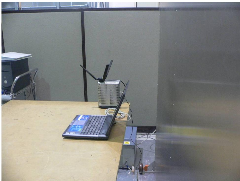
**Radiated Emissions - Front View**
