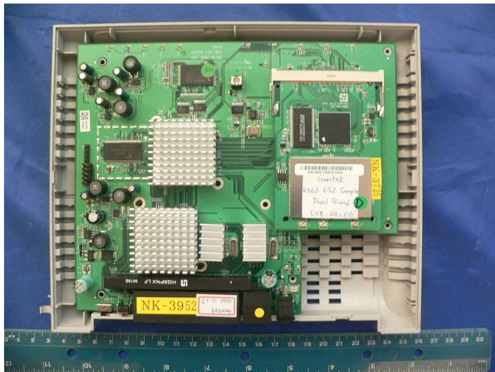
**EUT – Main Board Assembly (Component Side View)**
