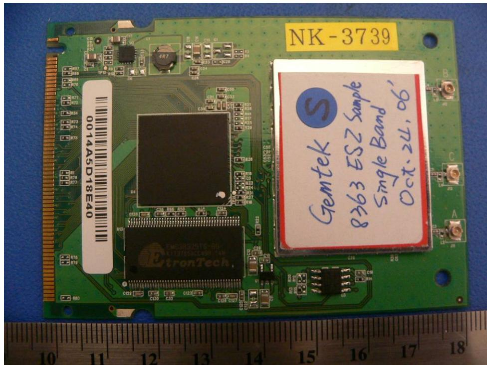
**EUT – RF Board Single Band without RF Shielding (Component Side View)**
