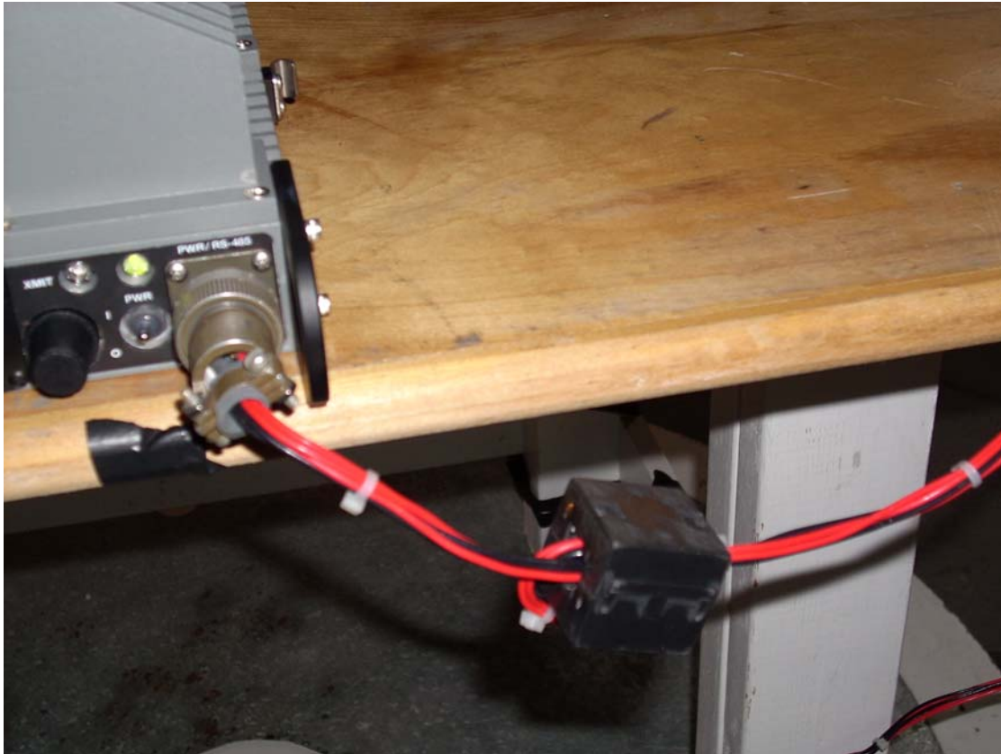
Figure 1 Ferrite modification required for compliance
