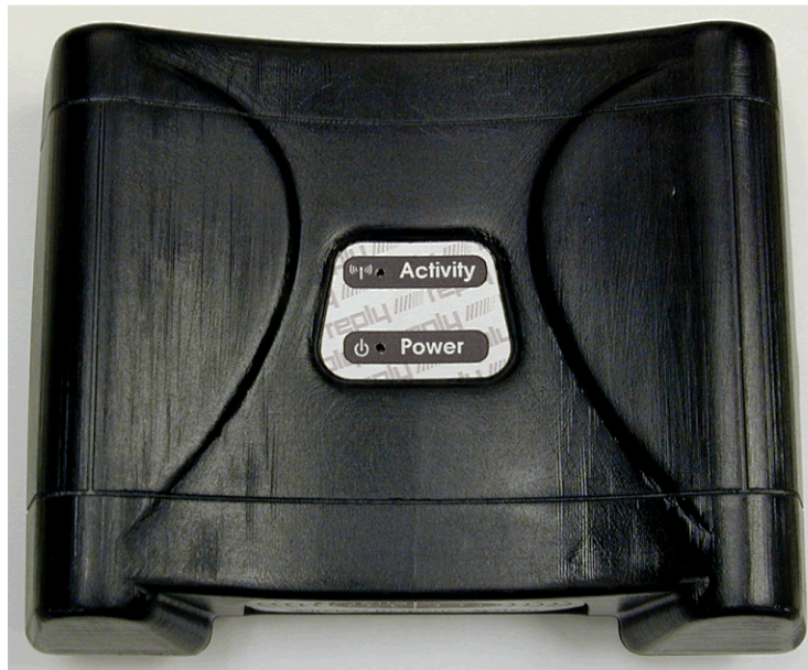
Reply WW housing – topside view. Note location of LED indicators.
