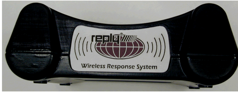
Reply WW housing – front side view. Note clamshell housing type.
