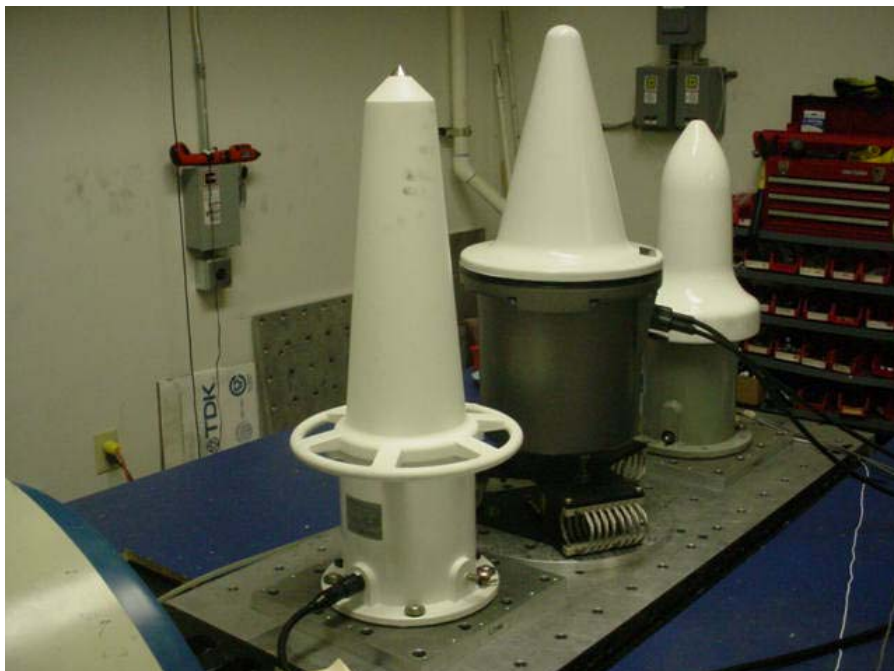
Photograph 4.16.3 Z Axis Vibration Test Setup
