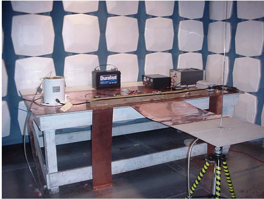
Photograph 4.20.1 RE102 Test Setup Front View
