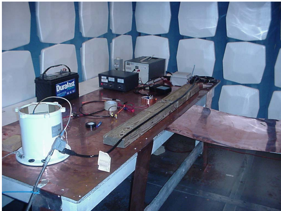
Photograph 4.20.2 RE102 Test Setup Side View
