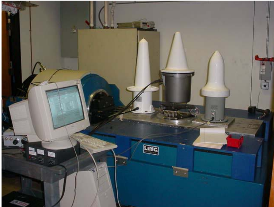
Photograph 4.16.2 X Axis Vibration Test Setup
