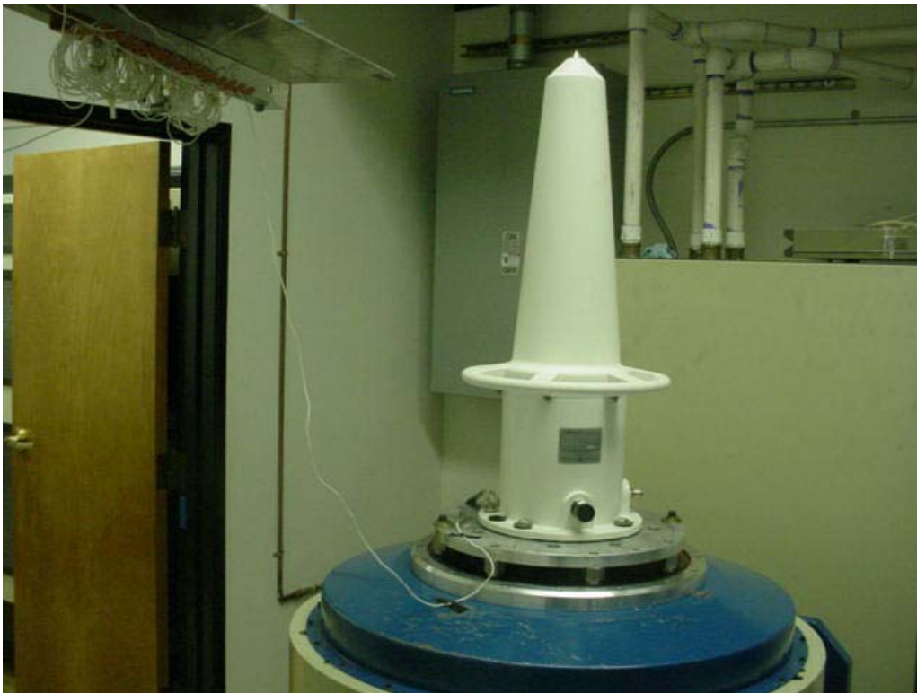
Photograph 4.16.1 Y Axis Vibration Test Setup
