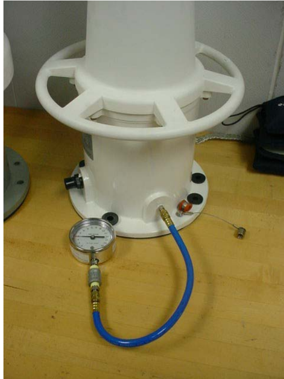
Photograph 4.18 Leak Test Setup
