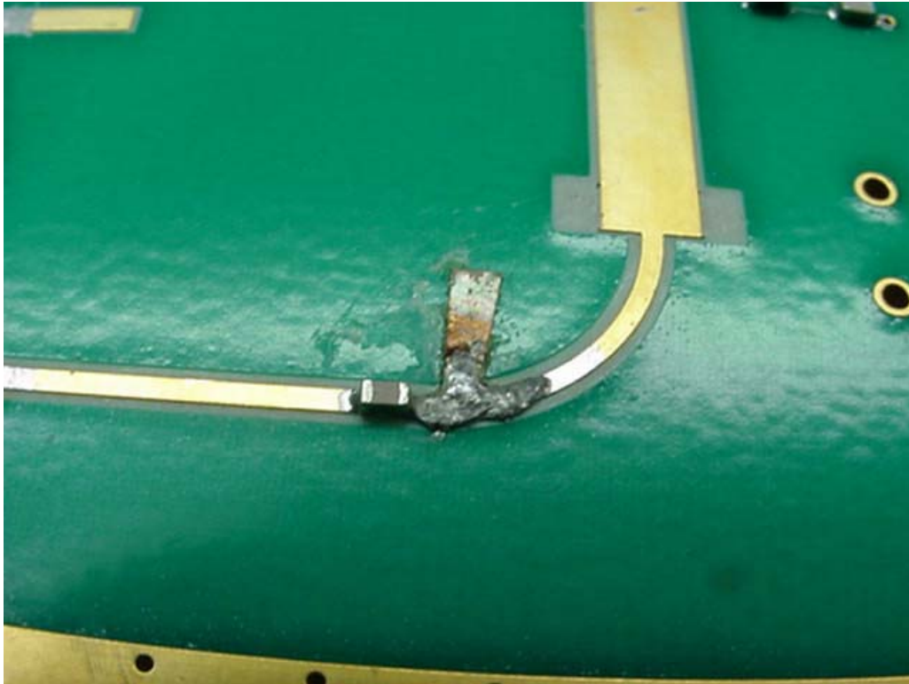
Photograph 4.22.2 SRF Cold Solder Joint
