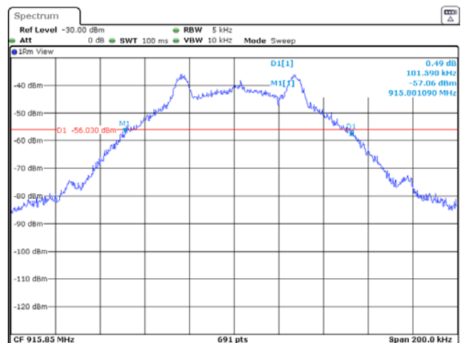
Plot 7.1.4 The 20 dB bandwidth test result at mid frequency
