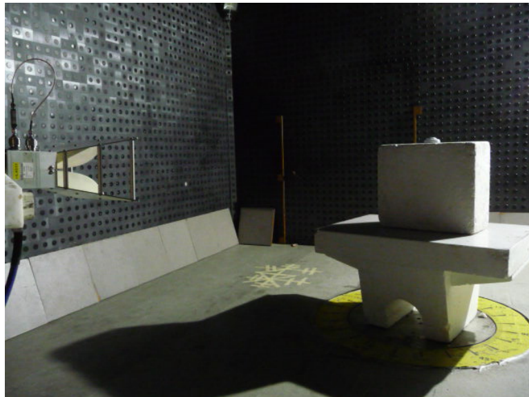
Photograph 8.1.2 Setup for radiated emission measurements above 1 GHz
