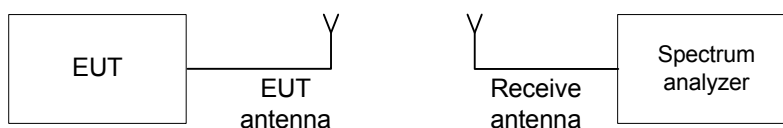
Figure 7.2.1 Carrier frequency separation test setup
