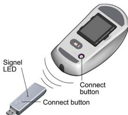
Step 1: Plug the dongle receiver into your computer. For the best performance, please plug the dongle receiver into the front USB port of your computer, or use the USB extension cable to place the dongle receiver 20cm away from monitor,
