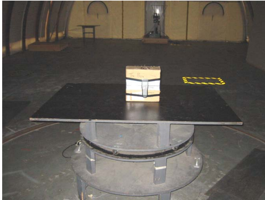
Radiated Spurious Test Setup, Front View
