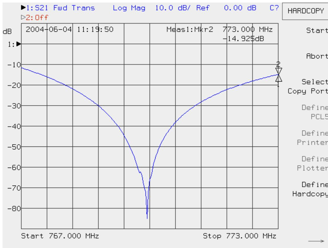
Two cavities notch (1000kHz frequency offset and in the receive band)
