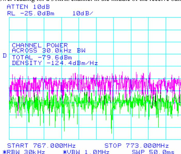
All the power channel read was below -78.5dBm/30kHz , after the correction of the 2.1dB inserted by the notch filter the absolute channel coupled power was found lower than -76.4dBm
