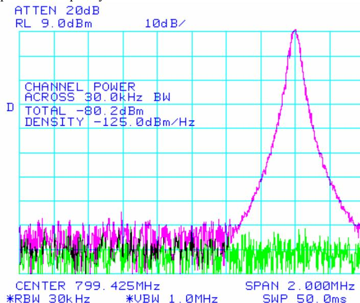
All the power channel read was below -75dBm/30kHz , after the correction of the 17dB (worst case) inserted by the notch filter the absolute channel coupled power was found lower than -58dBm
