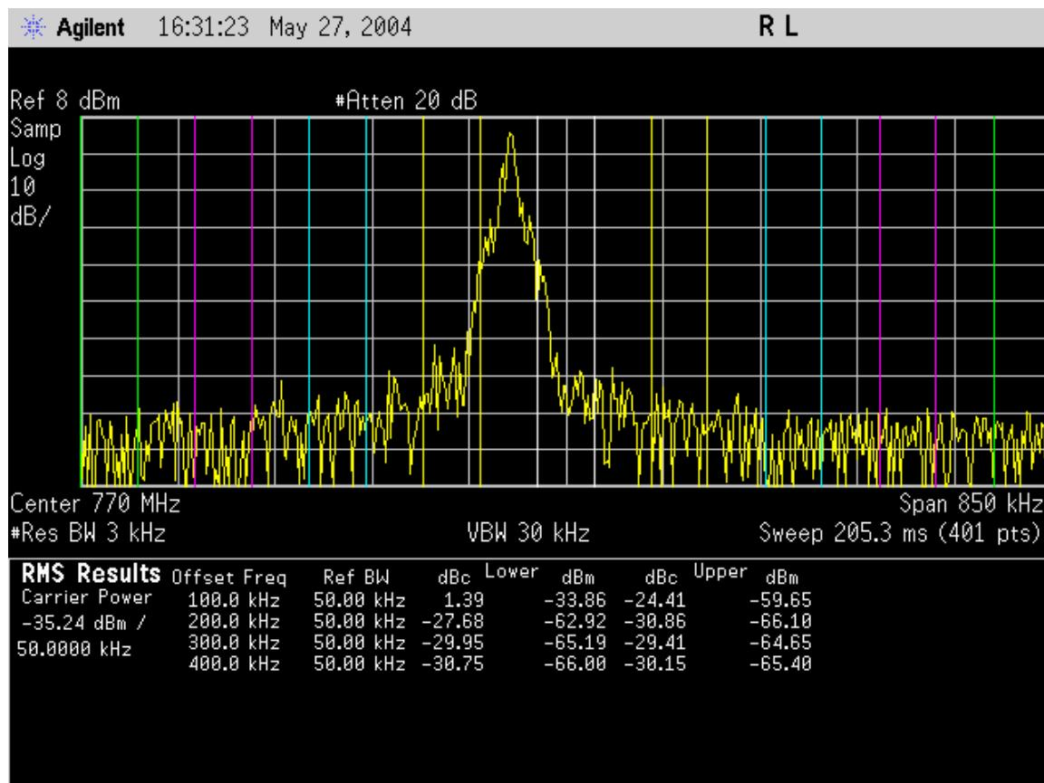
UUT in right channel (181) of the 150kHz 3-contiguous 50 kHz channels 179, 180, 181.
