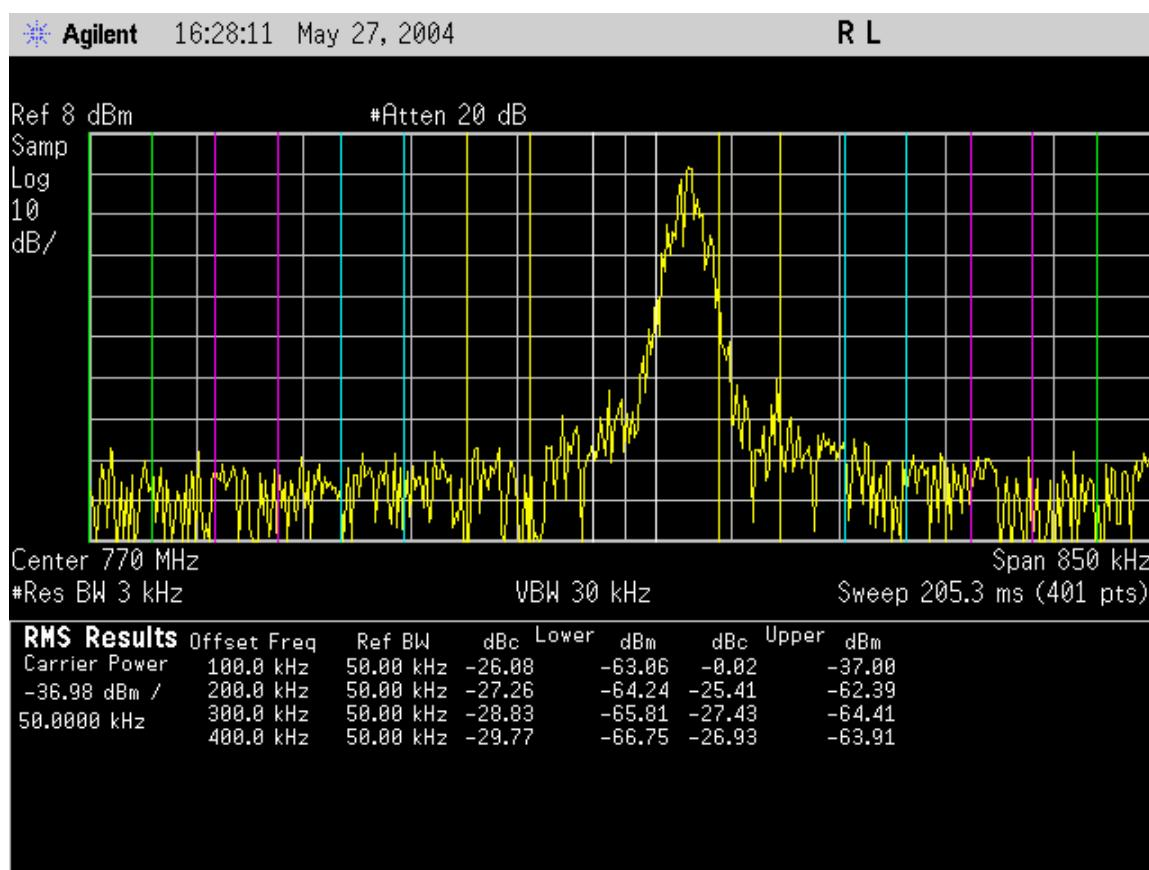
50 kHz channel (non-aggregated) adjacent channel coupled power.
