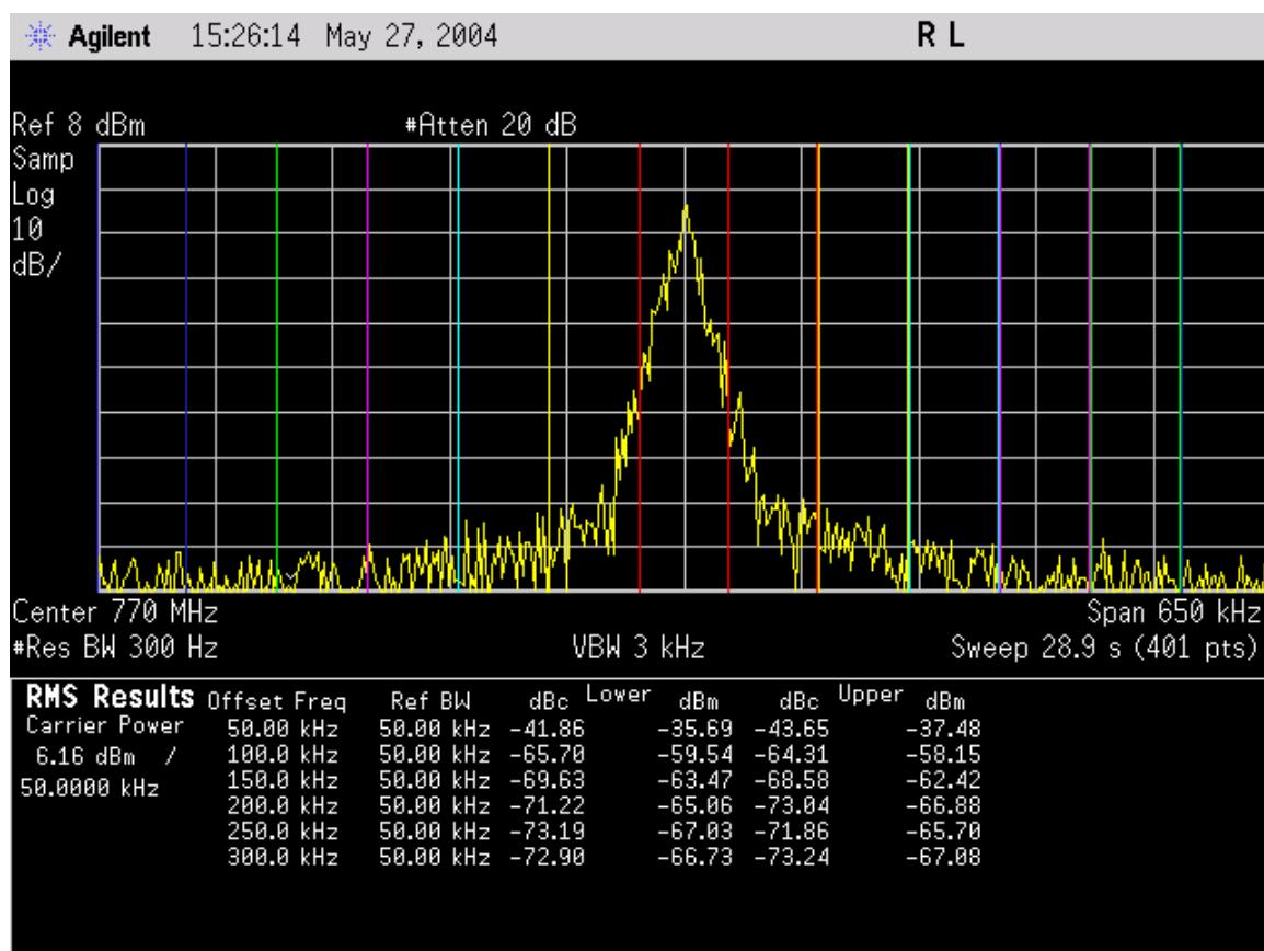
**Power Levels at frequency offsets >600kHz (90.534(b)(3))**
