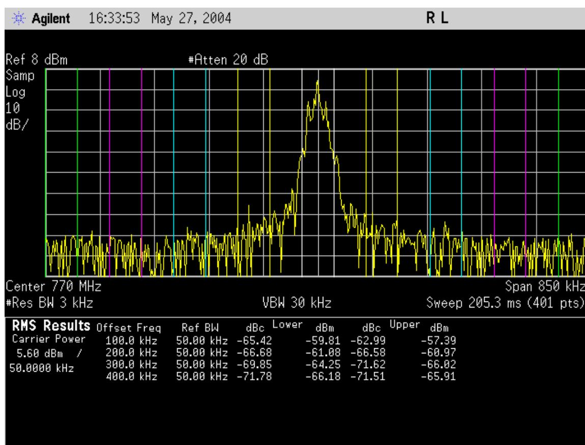
UUT in left channel (119) of the 150kHz 3-contiguous 50 kHz channels 119, 120, 121.
