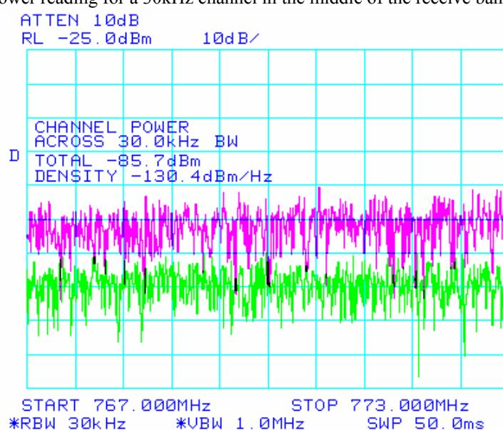
All the power channel read was below -82.3dBm/30kHz , after the correction of the 2.1dB inserted by the notch filter the absolute channel coupled power was found lower than -80.2dBm
