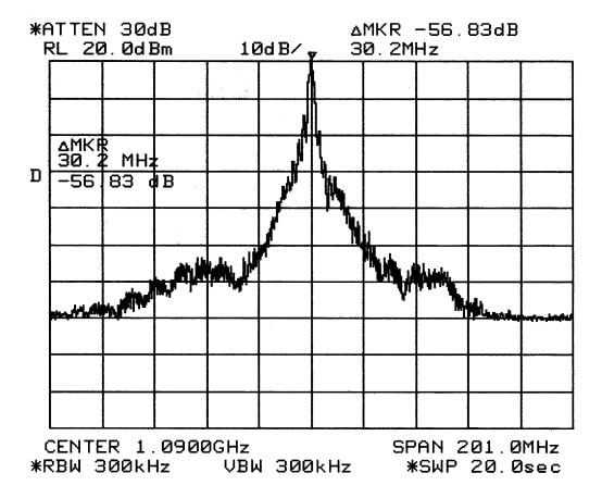
The measurement above was made in response to a request by the FAA's spectrum office after reviewing the submittal data. The marker is set to 30 MHz, which is the 250% BW point for 12 MHz authorized BW. Since we are requesting a 14 MHz authorized BW, the limit is actually 35 MHz. The measurement was therefore repeated and annotated accordingly as shown on the next page.
