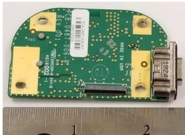
Communications Control Board - Bottom Side (all devices)
