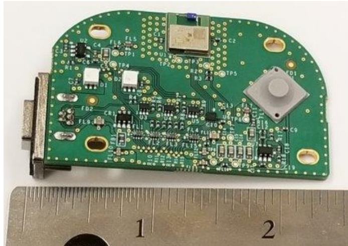
Communications Control Board - Top Side (all devices)
