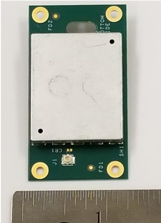
External Filter Board - Bottom and Top Sides (IMRB-EXT only)
