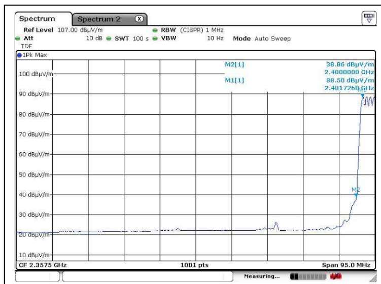
Lower edge (Bluetooth 3.0, Average measurement, hopping mode)
