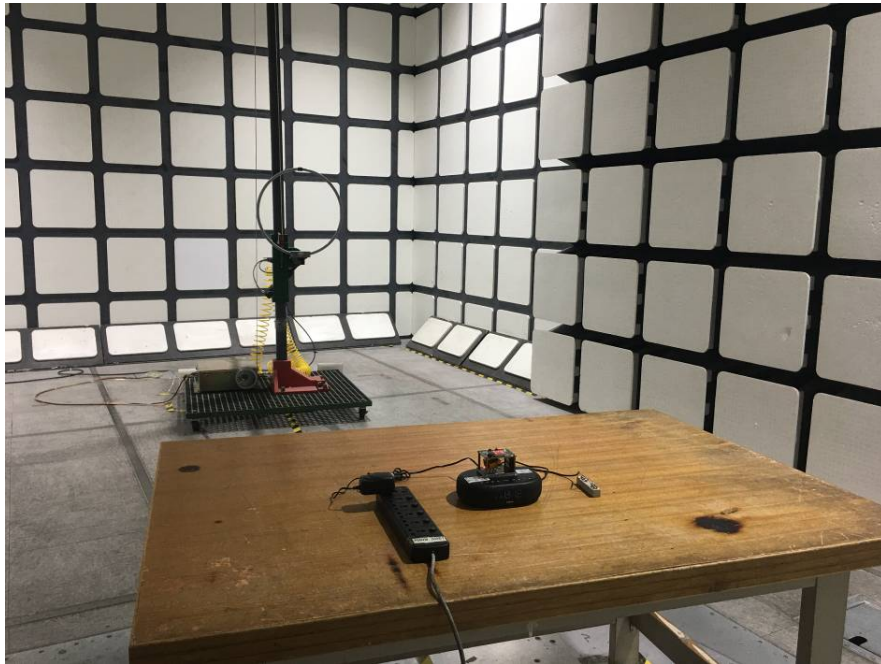
Radiated Emissions View (9 kHz ~ 30 MHz)
