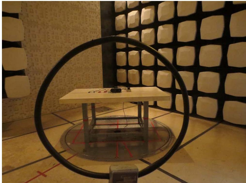
**Radiated emission test photos**
