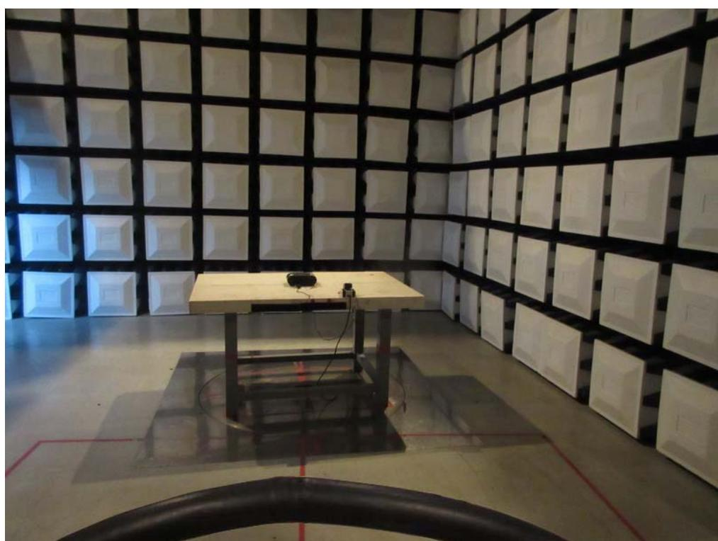
**Radiated Emission test photos****30MHz to 1000MHz**
