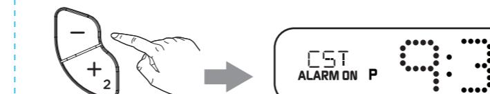
Press and release the **TIME ZONE** button to confirm time zone setting.
