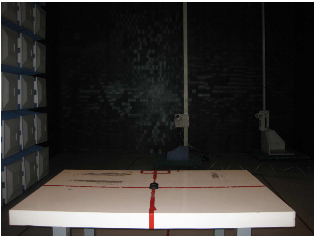
Photograph 4: Set-up for Radiated Emissions (18GHz-26GHz)
