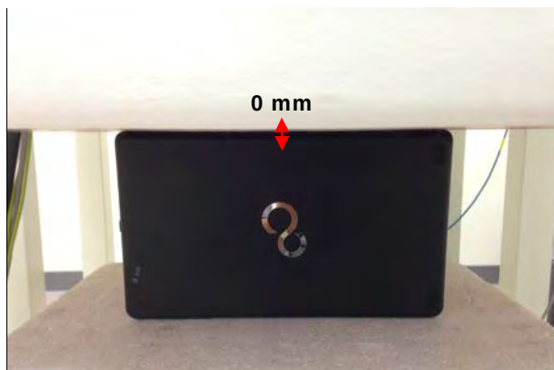
Fig.5 Left side to flat phantom
