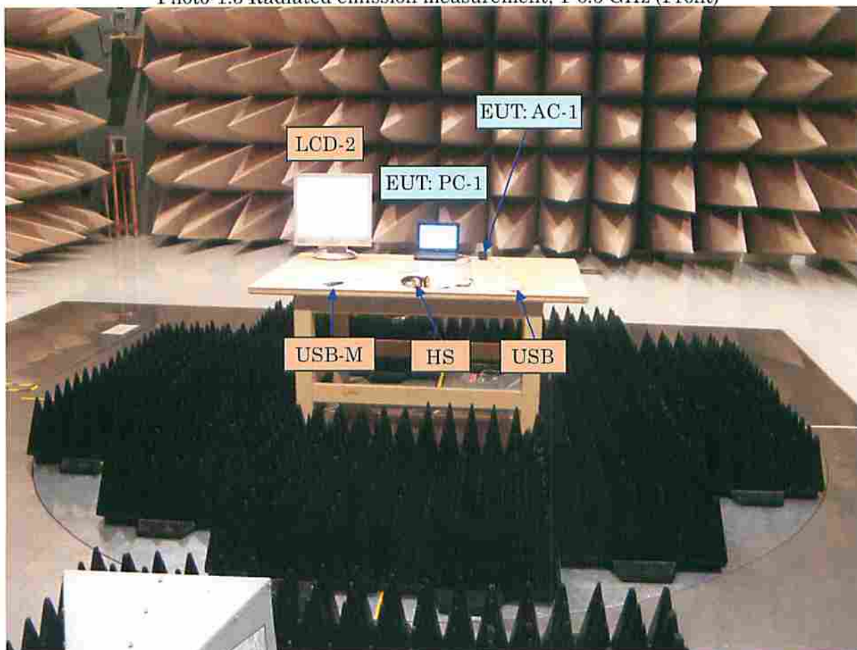
Photo-1.3 Radiated emission measurement: 1-6.5 GHz (Front)
