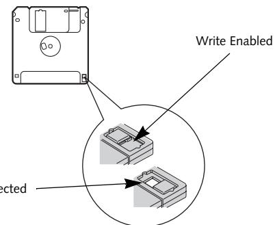
Figure 4-5. Floppy Disk Write Protect
