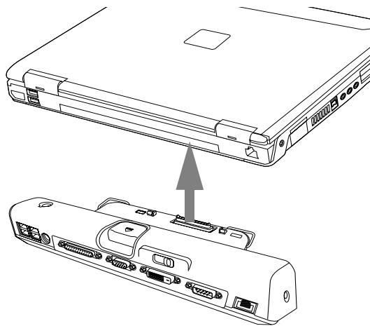
**Figure 4-13. Attaching the Port Replicator****LOCKING THE PORT REPLICATOR**
