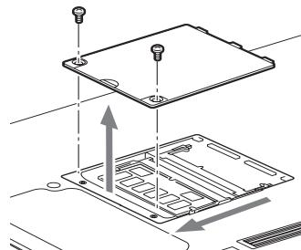
Figure 4-7. Opening the Memory Upgrade Compartment
