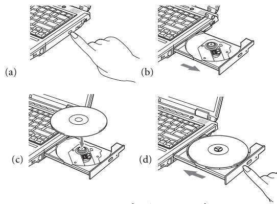
Figure 4-3. Loading/Ejecting Media
