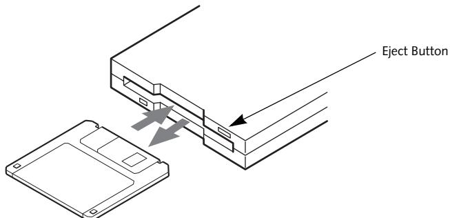
Figure 4-4&gt;Loading/Ejecting a 3.5" Floppy Disk
