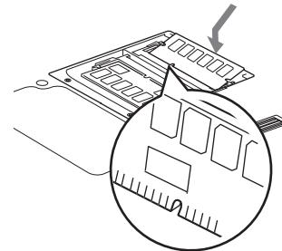
Figure 4-8. Installing a Second Memory Module
