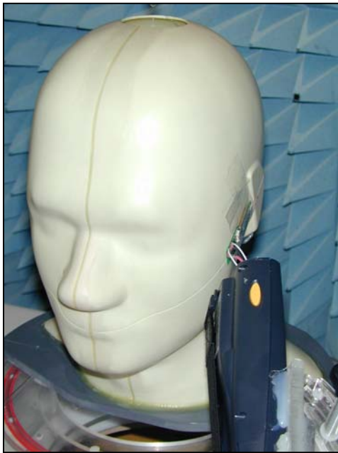
Figure 36. Positional photograph of the BTM210 Touch Position Left Cheek Module facing against SAM Phantom
