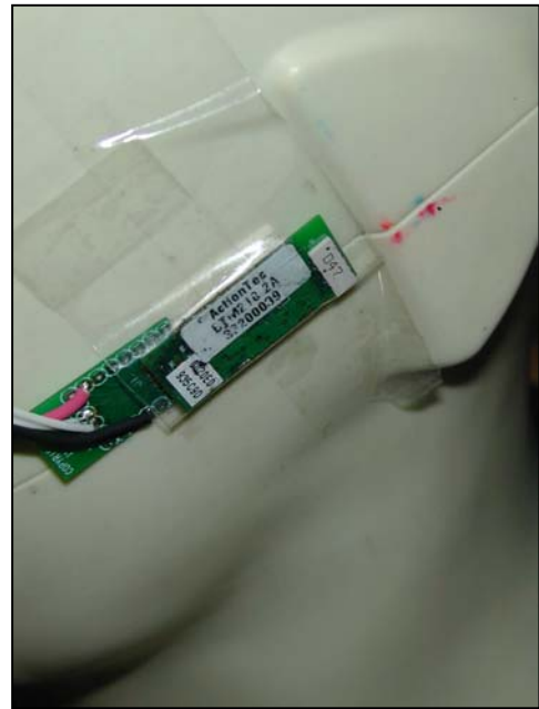
Figure 37. Positional photograph of the BTM210 Touch Position Left Cheek Module facing against SAM Phantom
