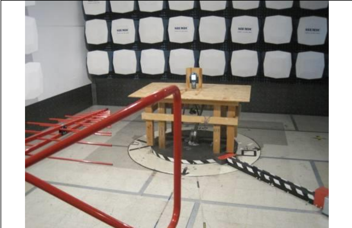
Radiated Emission Test Setup (30MHz – 1GHz) - Front View
