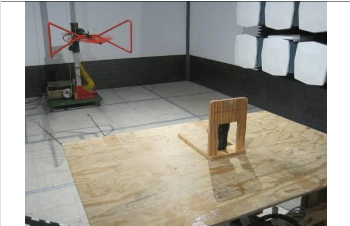
Radiated Emission Test Setup (30MHz – 1GHz) – Rear View
