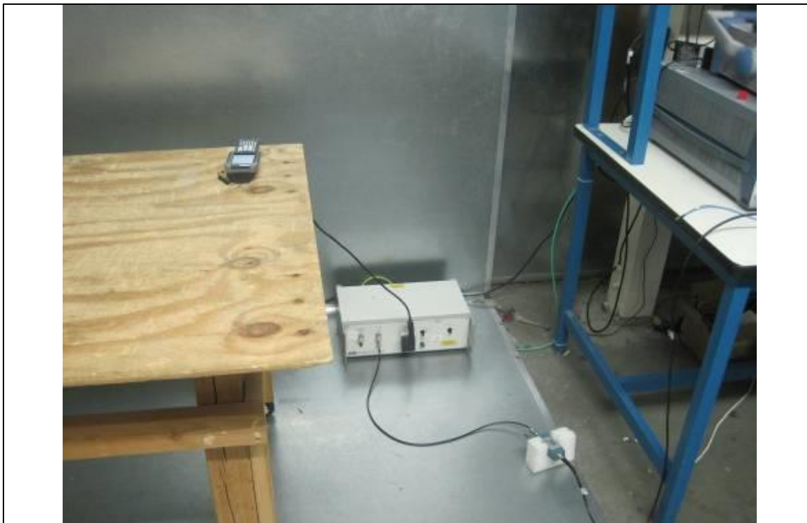
Conducted Emission Test Setup – Front View
