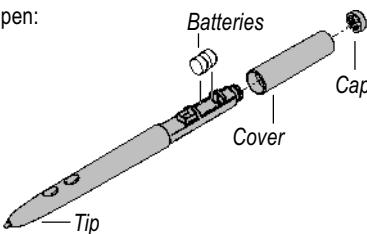
**Note:** You can operate the pen without batteries by connecting it to the tablet with the pen cord. This also keeps the pen tethered to the tablet, making it less likely to be lost. Instructions are included with the pen.
