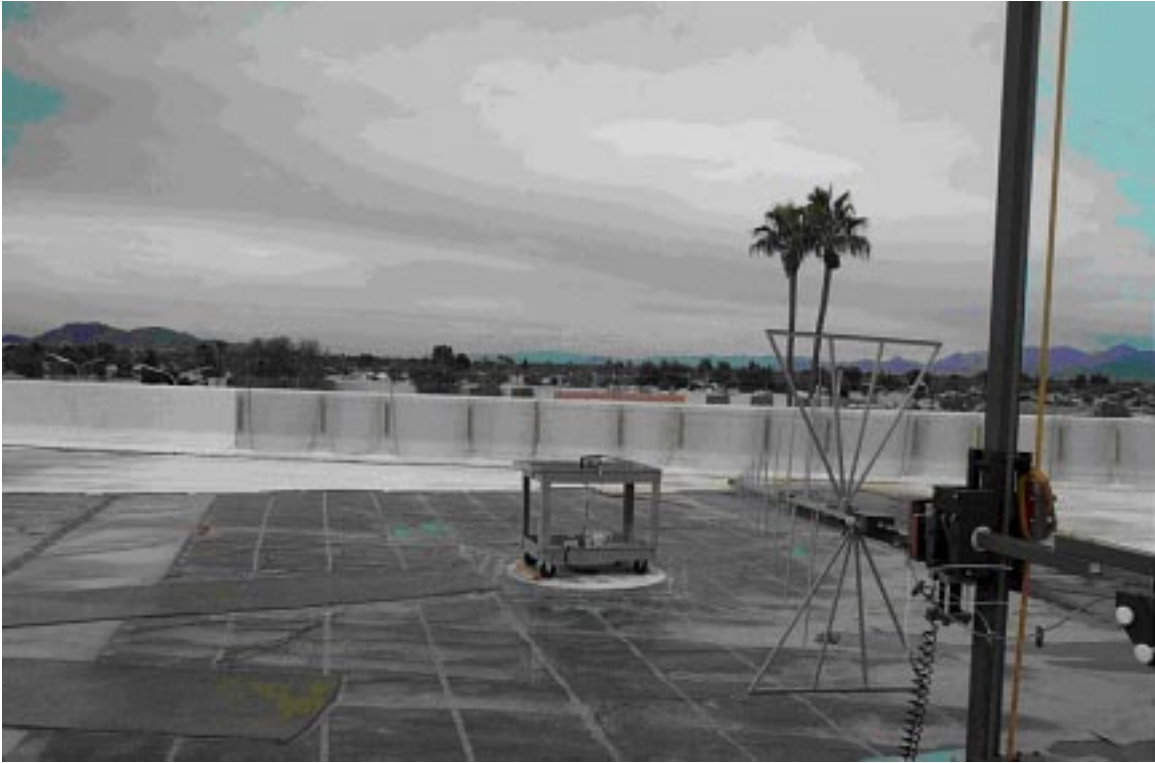
Figure C – 1 Radiated Spurious Emissions Test Setup, OATS
