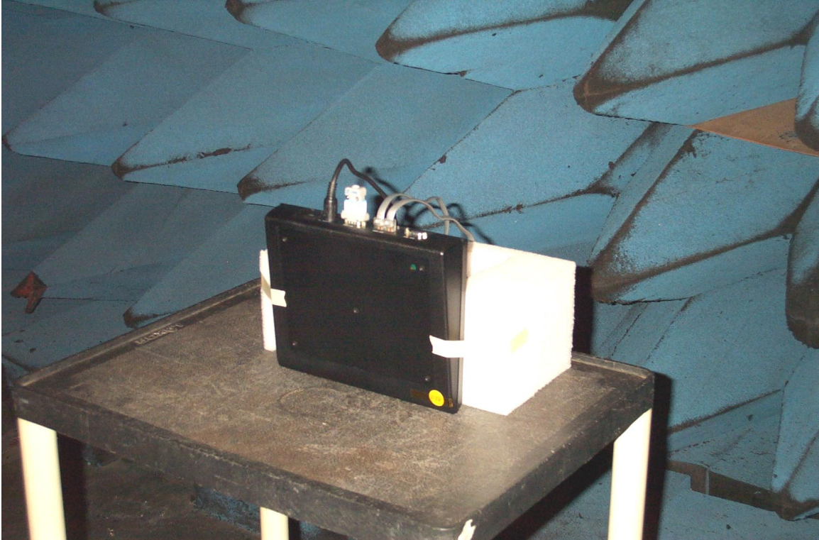
Figure D – 3 Radiated Spurious Emissions Prescan Test Setup, Chamber
