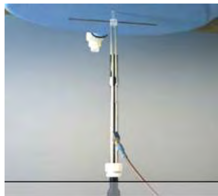
Photograph of the dipole Antenna
