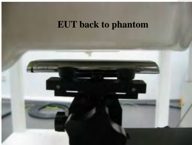
Fig.8 Body worn- EUT back to flat phantom and distance between flat phantom and mobile phone is 1.5 cm
