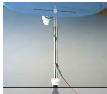
Photograph of the dipole Antenna
