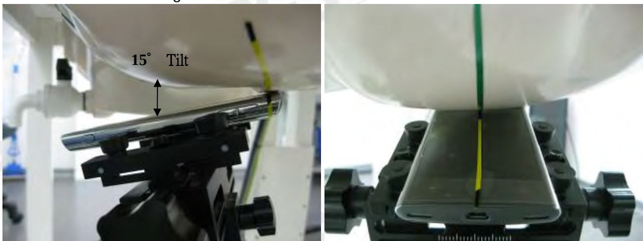
Fig.6 Left Head Section / Ear-Tilt Position(15°)
