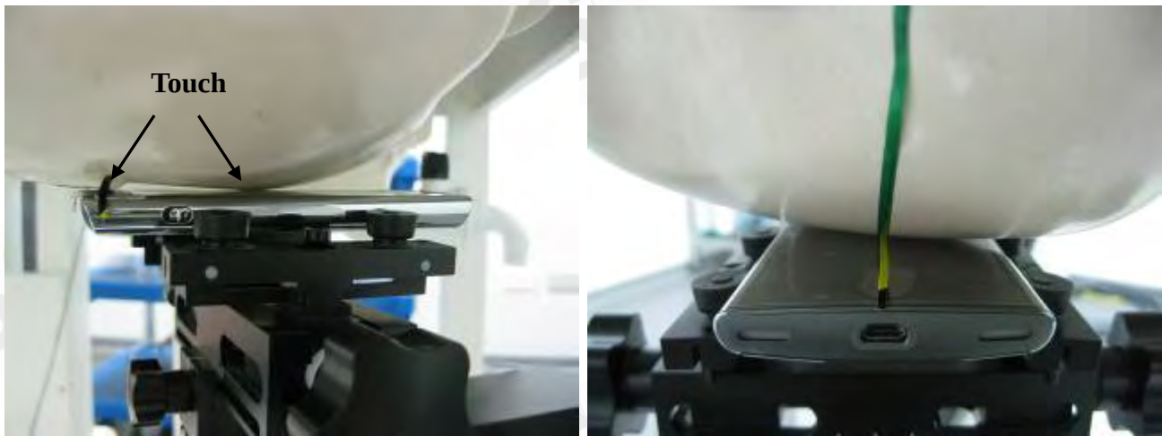
Fig.3 Right Head Section / Cheek-Touch Position
