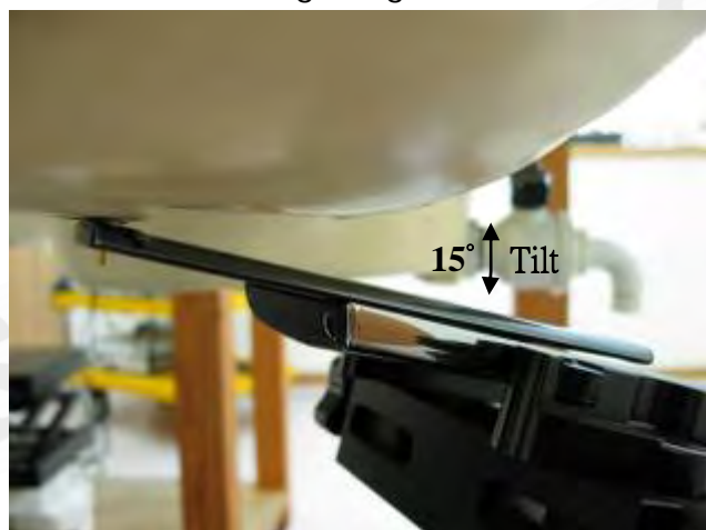
Fig.8 Right Head Section / Ear-Tilt Position(15°)_ Slider on
