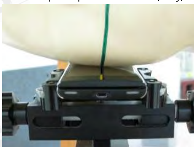
Fig.3 Right Head Section / Cheek-Touch Position_ Slider off
