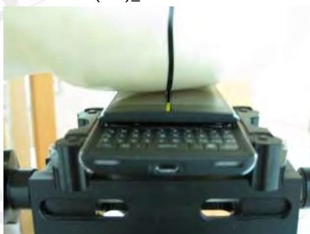
Fig.9 Left Head Section / Cheek-Touch Position_ Slider on
