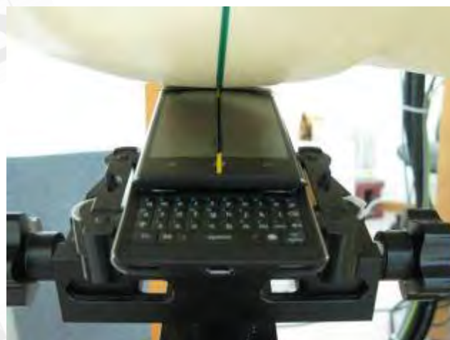
Fig.8 Right Head Section / Ear-Tilt Position(15°)_ Slider on
