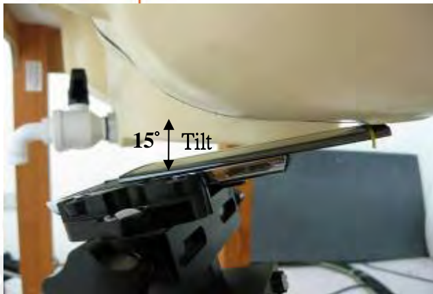
Fig.10 Left Head Section / Ear-Tilt Position(15°)_ Slider on
