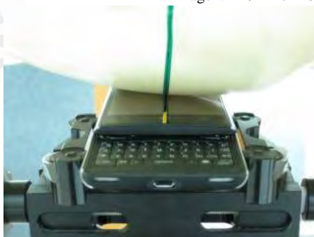
Fig.7 Right Head Section / Cheek-Touch Position_ Slider on
