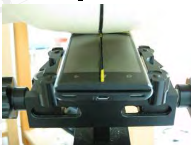
Fig.6 Left Head Section / Ear-Tilt Position(15°)_ Slider off
