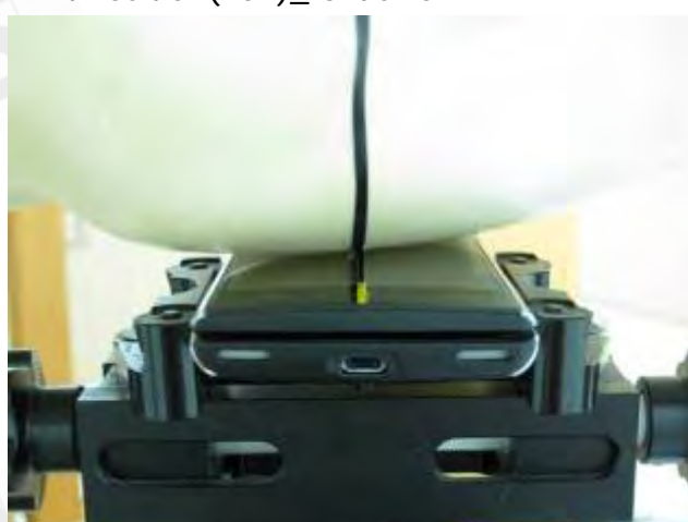
Fig.5 Left Head Section / Cheek-Touch Position_ Slider off
